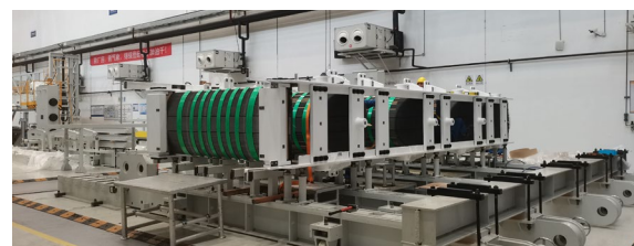
200 Tons Core Stacking And Turning Table
