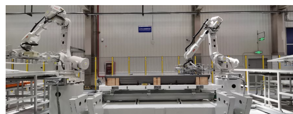
Automatic Core Stacking Robot
