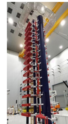
3000kV Impulse Voltage Generator
