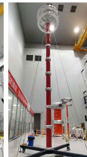
500kV Power-frequency Withstand Voltage Test Equipment
